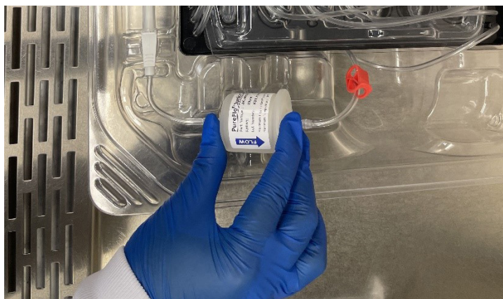
Figure 76. In-line filter lifted from the retention snap
