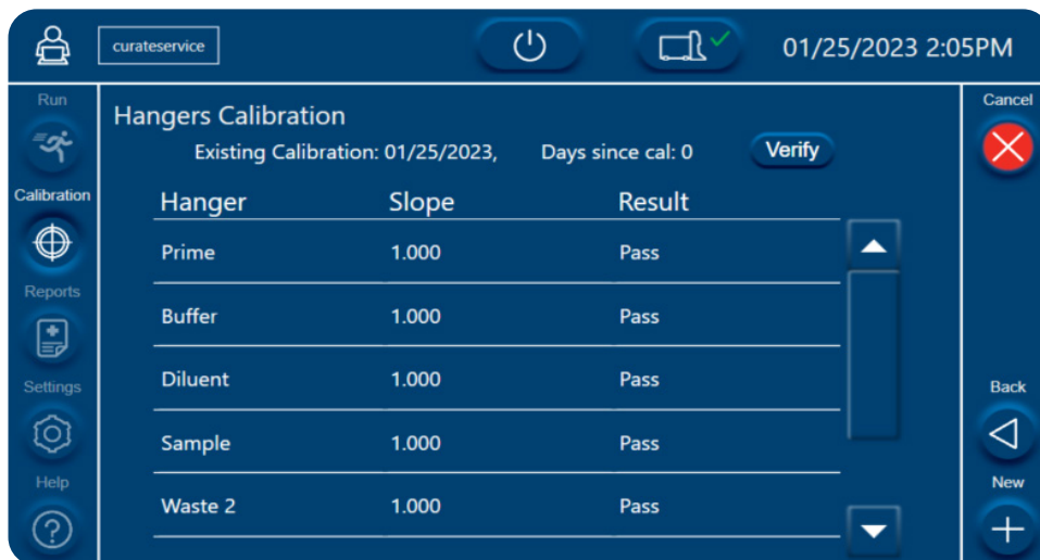
Figure 107. Hangers Calibration screen showing slopes and results
