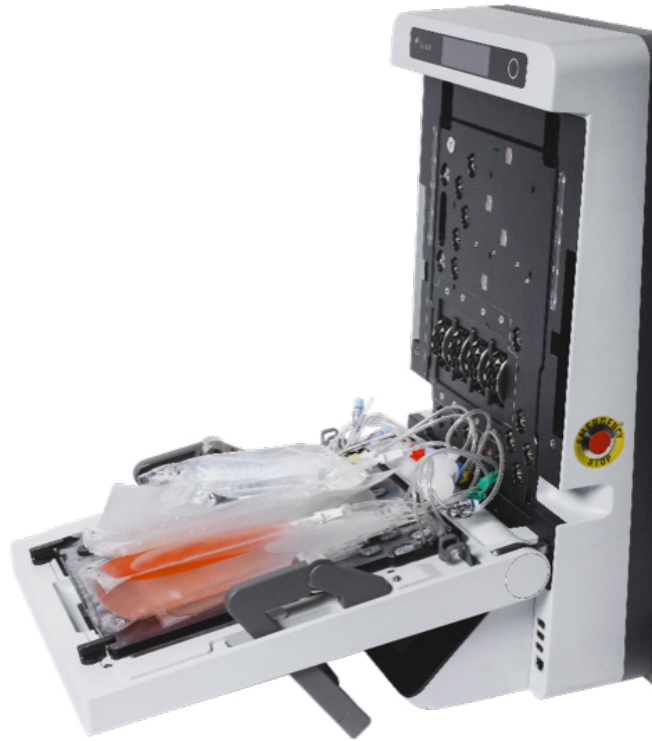
Figure 85. Open Curate Instrument door with cassette and bags
