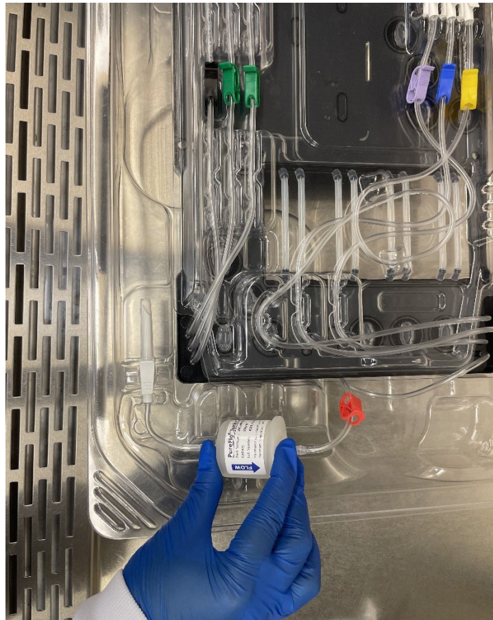
Figure 71. In-line filter lifted from the retention snap
