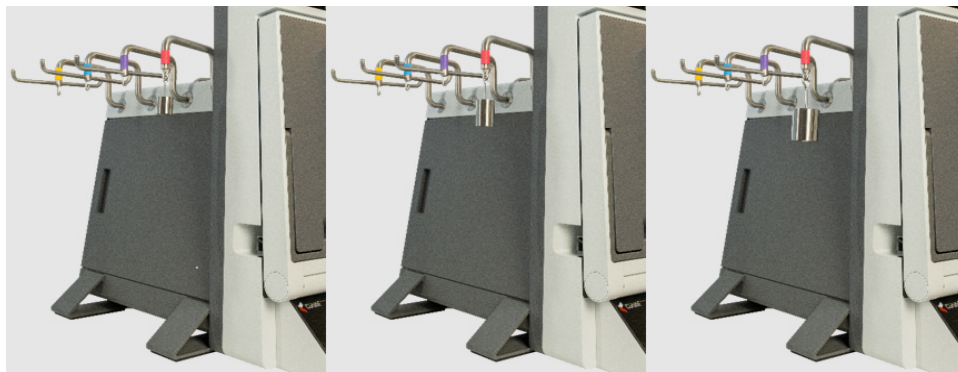
Figure 101. Calibrating with standard weights
