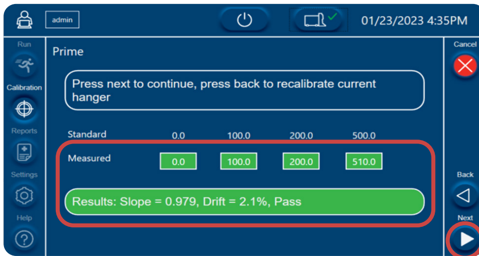
Figure 106. Prime screen with green value boxes, indicating successful calibration
