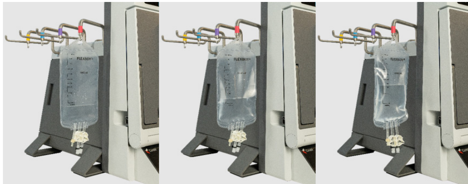
Figure 102. Calibrating with bags of water
